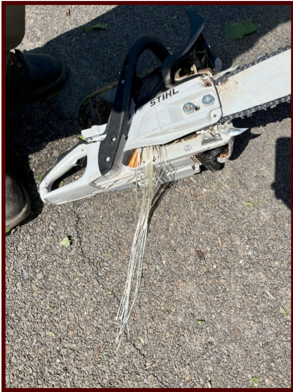
Figure 4. Long Kevlar fibers hanging from out of the clutch cover.
