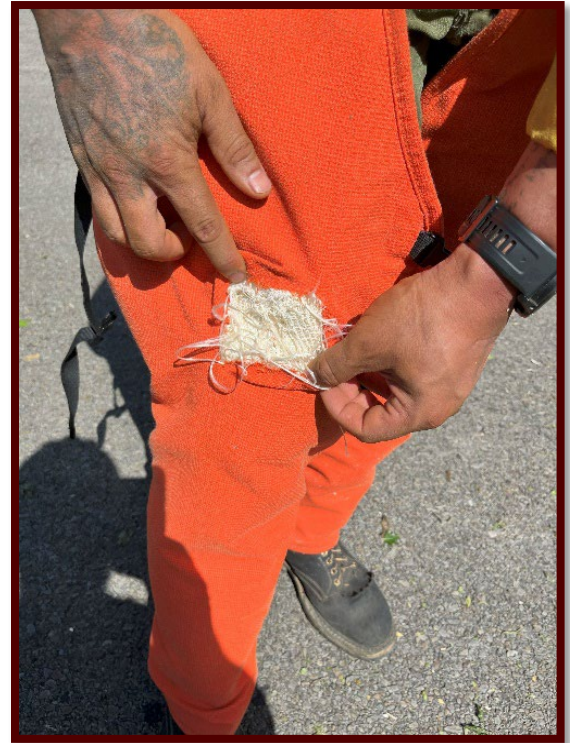
Figure 3. After opening the cut, it can be seen how the chainsaw had gone through the outer shell and the first layer of Kevlar and stopped in the second layer of Kevlar.
